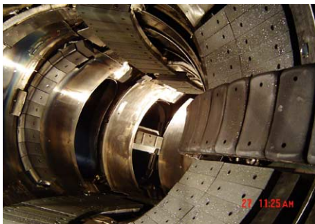
Fig. 1. Poloidal and toroidal water-cooling limiters in the HT-7 tokamak.
